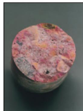
Concrete Core Showing Advanced ASR
