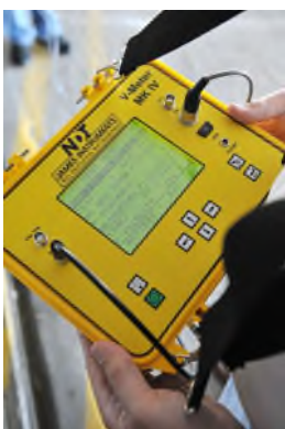
V-Meter MK IV™ Showing Elapsed Time
